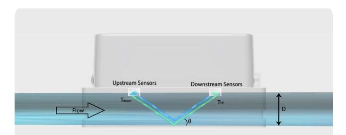
$$V = \frac{MD}{\sin 2\theta} \times \frac{\Delta T}{T_{up} \cdot T_{down}}$$
